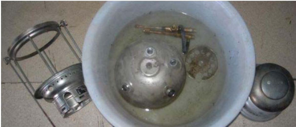
Pic. 3: The bucket with the main parts in citric acid
