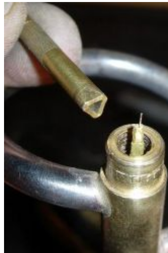
Pic. 13: needle mounting
