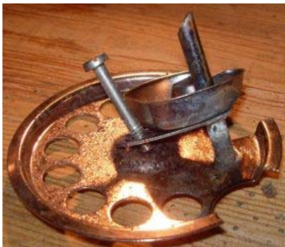
Pic. 18: Centre bottom plate, centre screw and pre-heater cup
