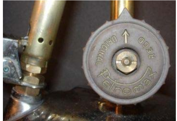
Pic. 48: Valve wheel in 'closed' position
