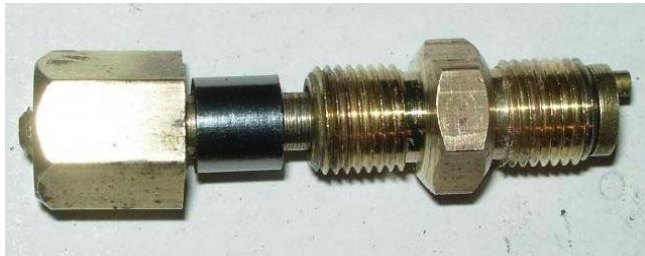
Pic. 45: A new graphite packing (#108) fitted
