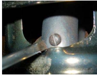
Pic. 36: Adjusting the mixing tube 'paddle'
