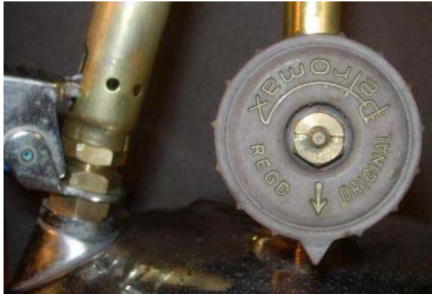
Pic. 47: Valve wheel in 'open' position
