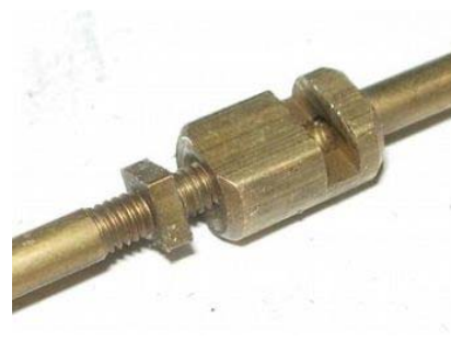
Pic. 16: Secure adjustment w. counter nut
