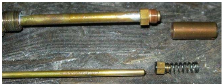
Pic. 40: Lower part of gen w. gen rod foot valve body, spring and seal
