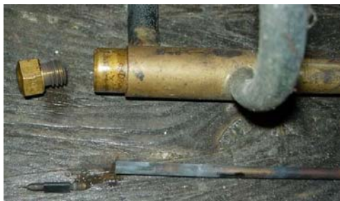
Pic. 39: Upper part of gen with nozzle and needle
