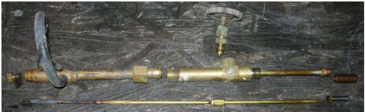
Pic. 38: Complete generator with rod, foot valve, main valve and nozzle with needle
