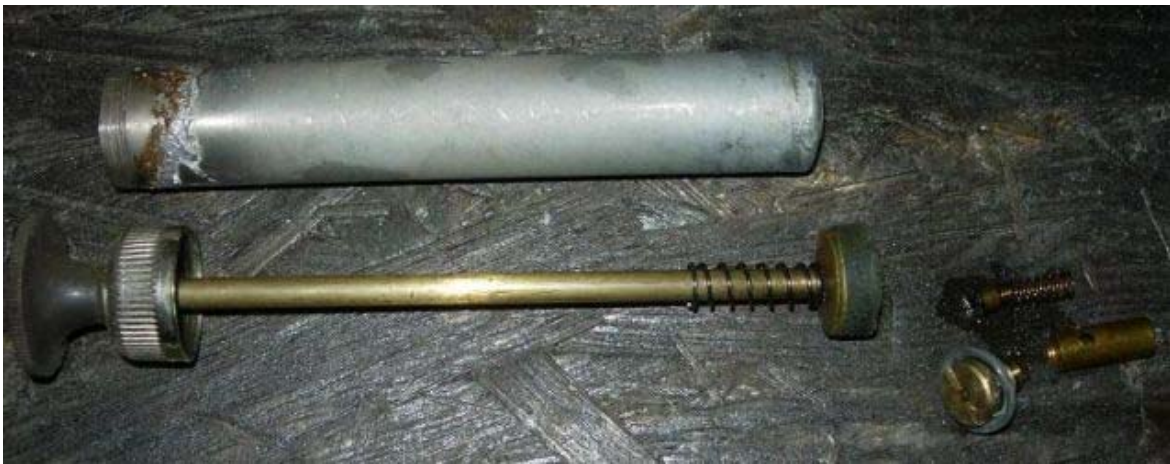
Pic. 51: Pump, pump body and pump check valve
