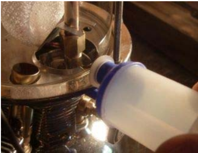
Pic. 27: Filling alcohol in the cup w. bottle
