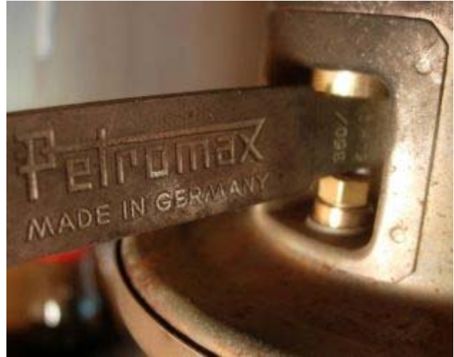
Pic. 25: Adjusting the mixing tube distance
