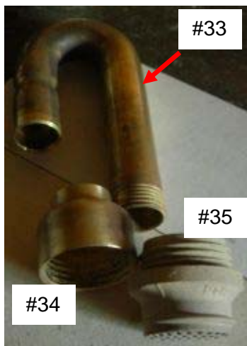
Pic. 21: Burner parts
