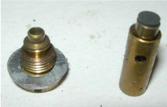
Pic. 49: Pump check valve disassembled
