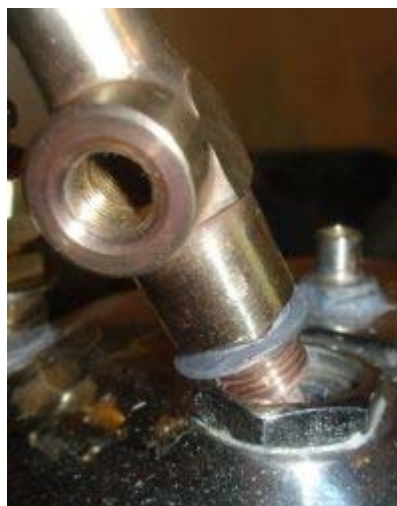
Pic. 11: Lower part of gen w. lead washer
