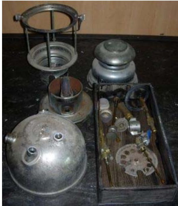
Pic. 2: Lantern completely disassembled into parts.
